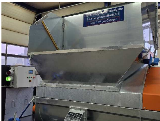
Feed hopper – Splash plates folded down for transport
