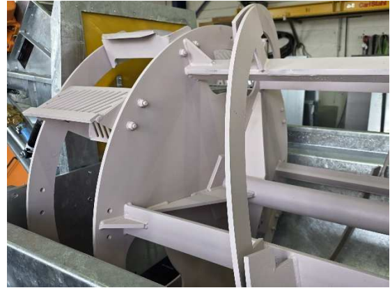
Helix and bucket elevator
