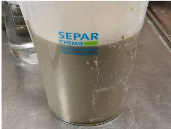
Bentonite suspension - untreated
