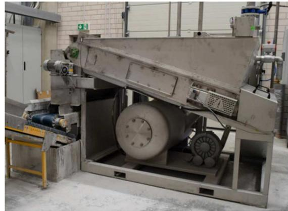
Vakuum belt filter in use
