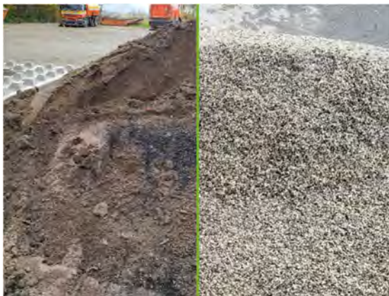
Mineral waste (left) becomes substitute building material (right)
