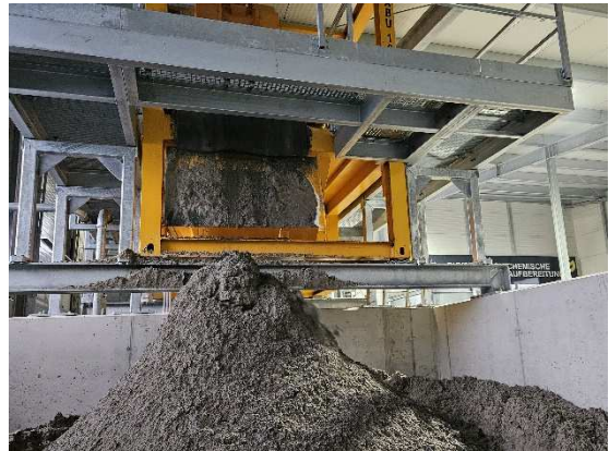
Fines separation for components >60 \mu\text{m}
