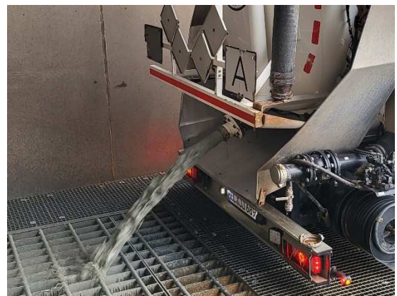
Emptying drilling fluid from silo vehicle
