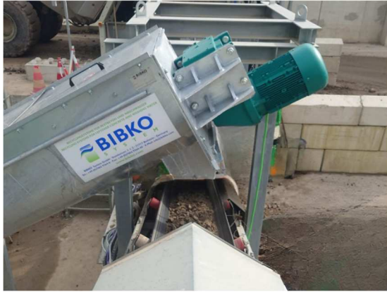
Screw conveyor with inclined belt
