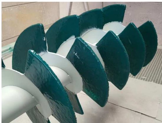
Conveyor screw with recesses and wear protection
