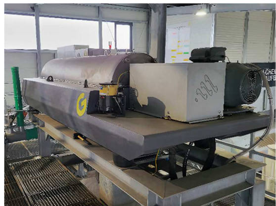
Process water recycling with centrifuge
