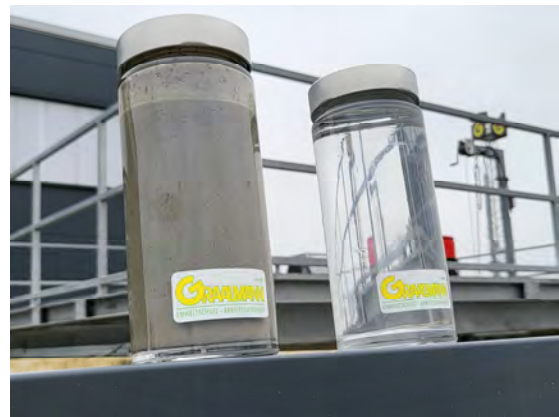
Drilling fluid (Input) | Centrate (Output)
