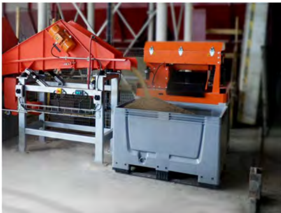
Material discharge with vibrating chute
