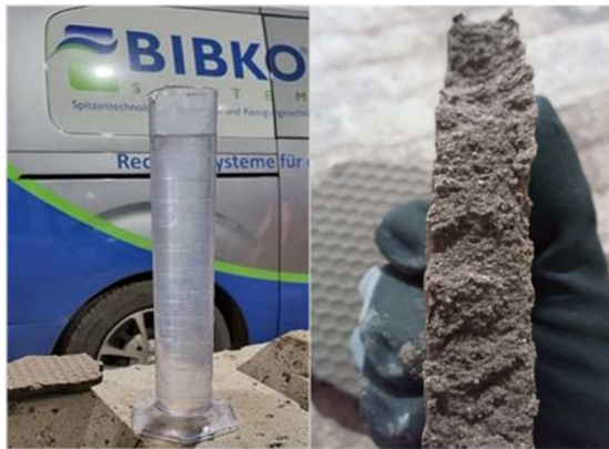
Filtrate/ filter cake after filtration with a filter press
