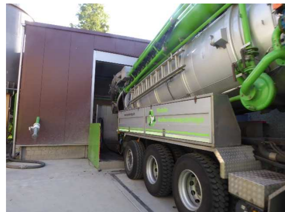
Suction/flushing vehicle during emptying
