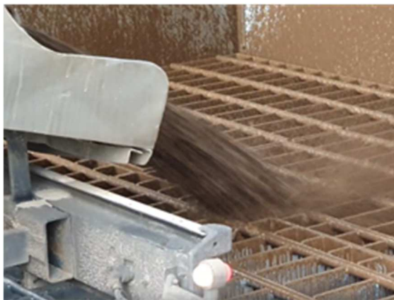
Emptying bentonite suspension
