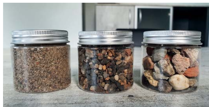
Recyceltes Material – gesiebt: 0...2/ 2...8 mm/ 8...16 mm
