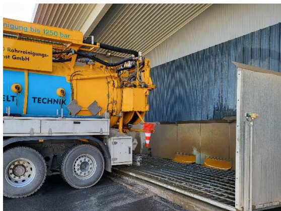
Sewer cleaning vehicle - emptying at recycling machine
