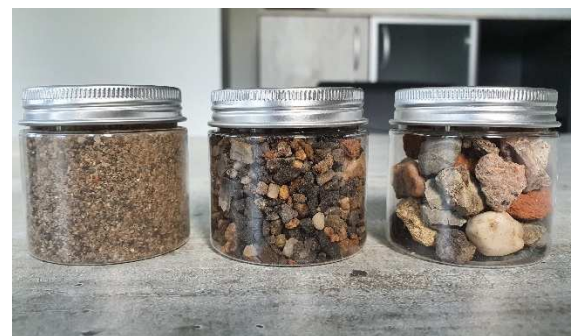
Recycled material - screened: 0...2/ 2...8 mm/ 8...16 mm
