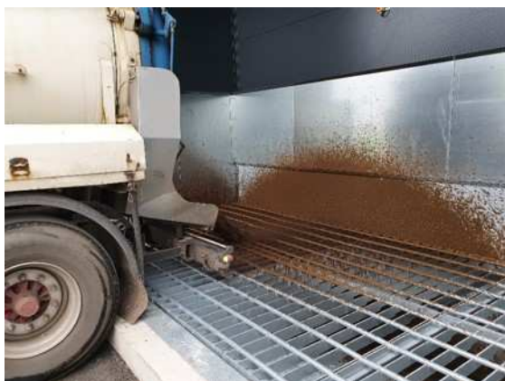
Material example: Bentonite suspension
