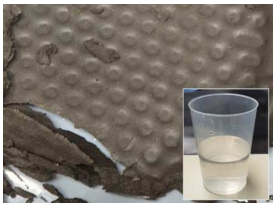
Filter cake/ filtrate after filtration
